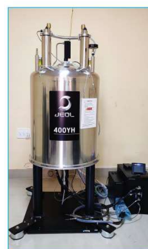
NMR SYSTEM Model/Make: Jeol, JNM-ECZ400S/L1, Japan
